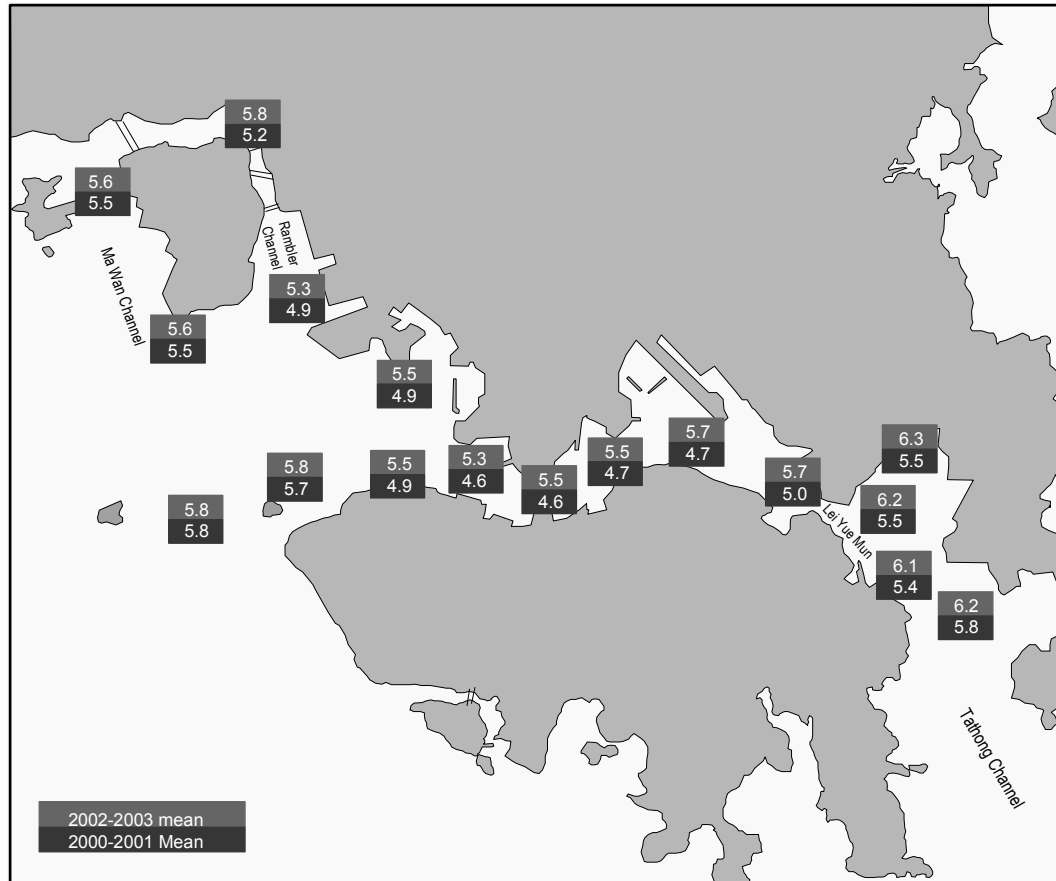
Figure 2 Map showing changes in dissolved oxygen (mg/L) at 17 stations in the HATS enhanced monitoring (comparison of mean difference between Jan 2002 – Dec 2003 and Jan 2000 – Dec 2001)
